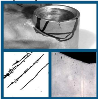
Fig 2.4.5 Cracks and Hot-Cracking
