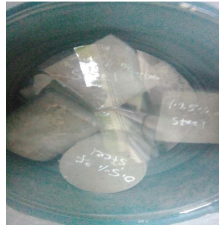
CUBE SPECIMENS STORED IN CURING TANK
