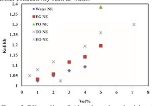
Figure 3. Effect of base fluid on thermal conductivity of nanofluid.
