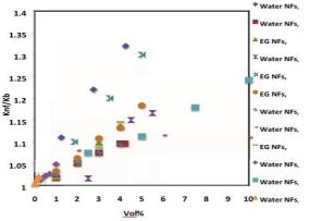
Figure 1. Effect of volume fraction of nanoparticles on ratio thermal conductivity of Al2O3-based nanofluids
