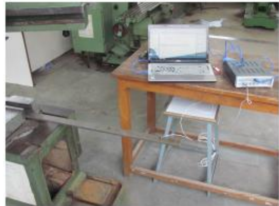
Figure 6: Experimental Set-up for Crack Detection of a Cantilever Beam with a Single Crack
