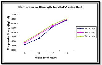
The above graph show variation of compressive strength with respect to concentration of NaOH at different molarities. As the concentration of NAOH increases the compressive strength also increases.
