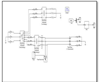
Fig-6 Voltage Sag condition in 3-phase system There is 3-phase fault is created in the three phase system which creates voltage sag problem in this system. The three phase fault is operated and controlled through external timer signal. The Simulation of this model shows that voltage Sag condition occurs at input side and the point of common coupling.
