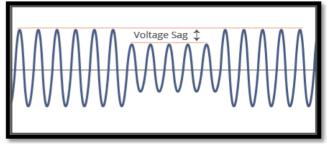
Fig.1- Voltage Sag condition
