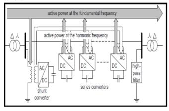
Fig 4 Active power exchange between DPFC converters
