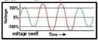
Fig.2-Voltage swell condition
