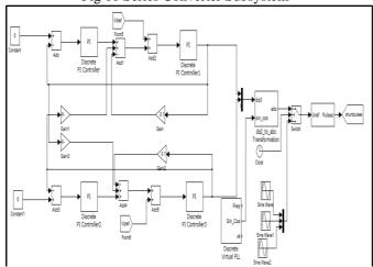
Fig.11 Shunt Converter Subsystem
