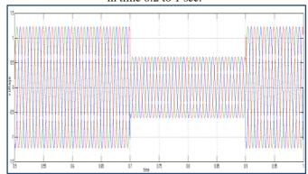
Fig 14 Waveform of voltage sag at source side in time 0.5 to
