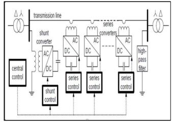
Fig.5 DPFC control block diagram
