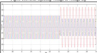
Fig.16 converter injecting voltage in fault sag
