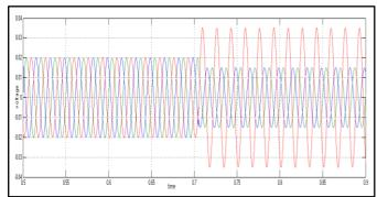
Fig.15 converter injecting voltage in voltage dip
