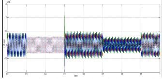
Fig 13 Waveform of voltage sag due to fault and source dip in time 0.2 to 1 sec.
