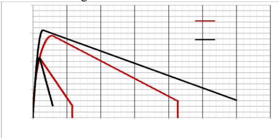
Figure 3.1 Comparison of stress-strain curves using two confinement models (Razvi and Modified Kent models) for the RC section 400C-2S4B-SM ( K_1 = 6.47 , K = 1.47 )
