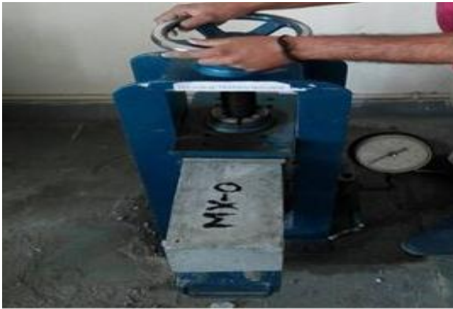
Fig. 2 TEST SET UP FOR BEAM
