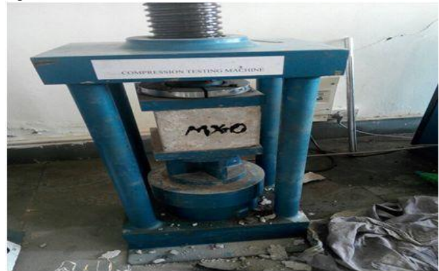
Fig. 1 CUBE UNDER COMPRESSION TESTING MACHINE (CTM)
