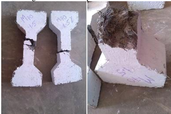
Fig.15: Failure of specimens 1.5% fibre
