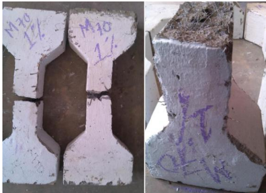
Fig.14: Failure of specimens 1% fibre
