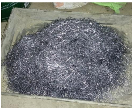
Figure – 1 Hooked end steel fibre
