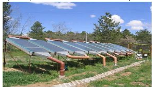
[Storage type solar air heater by Huseyin Benli]
