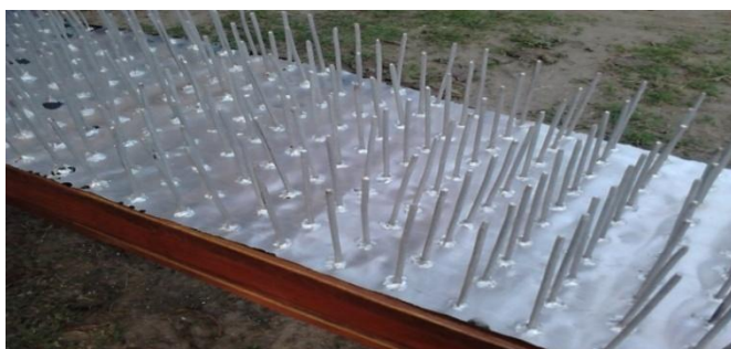
[Aluminium fins welded on bottom surface of absorber plate]
