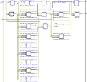
Figure 6 8-bit ALU MUX RTL View
