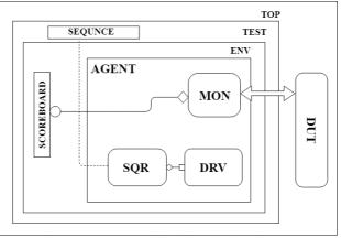
Figure 8 UVM Verification Block Diagram
