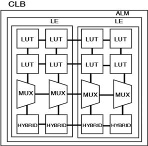
Figure 4 In FPGA CLB Architecture
