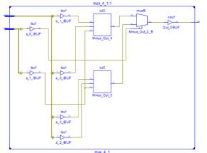
Figure 3 Using LUT and MUX Hybrid to Design 4:1 MUX
