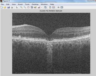
Figure 5.4 Shows the KUAN Filter Image Kuan filter were the earliest filters working directly on the intensity of the image using local statistics and is based on the minimum mean square error (MMSE), which produce the speckle free image governed by the relationship
