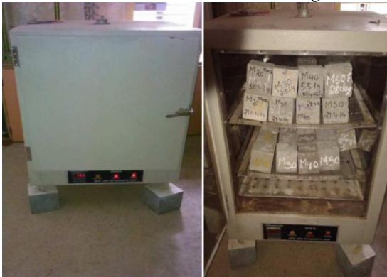
Fig 1. Electric oven with specimens kept for thermal cycles
