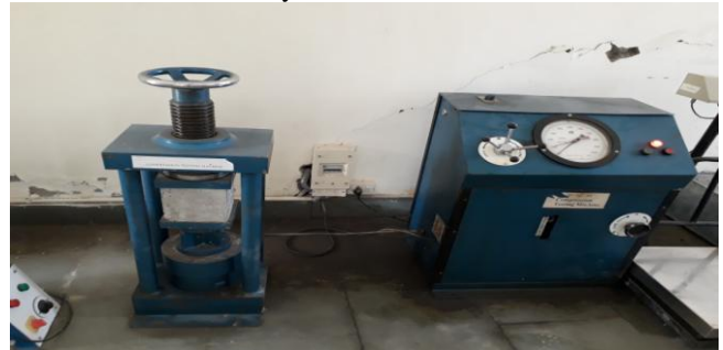
Fig. No.4.1: Testing of Cube
