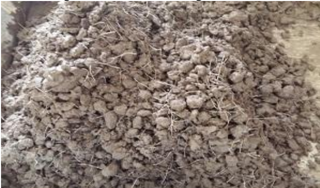
Fig 3.2 Addition of Glass Fibre into Mix
