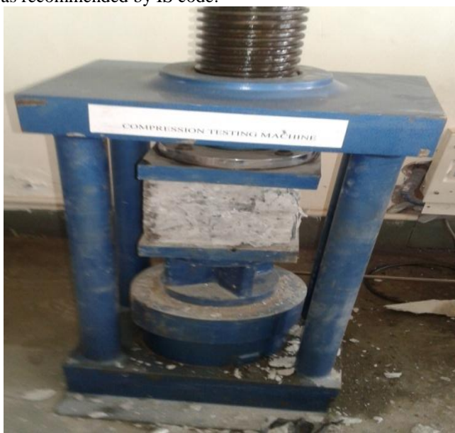
Fig. No.4.1: Testing of Cube
