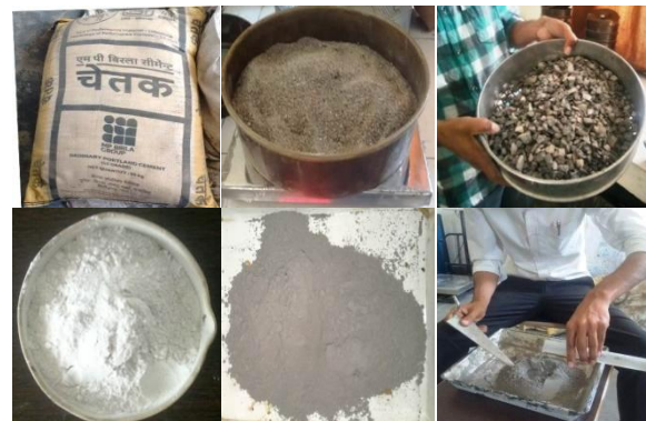
FIG. (I) CONCRETE INGREDIENTS AND ADMIXTURES
