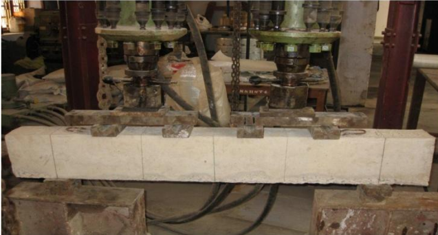
Fig 5.19 Loading arrangement beam CB1
