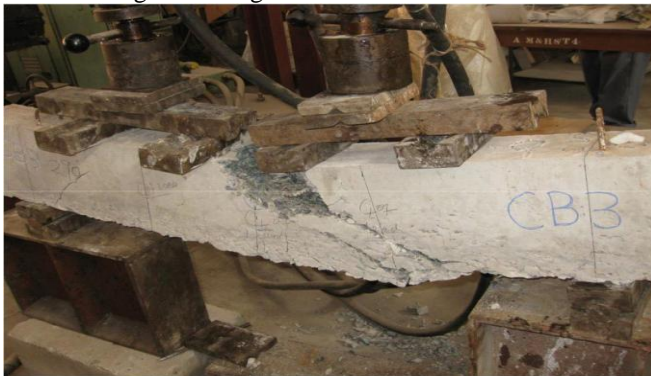
Fig.5.27 Failure of beam CB3
