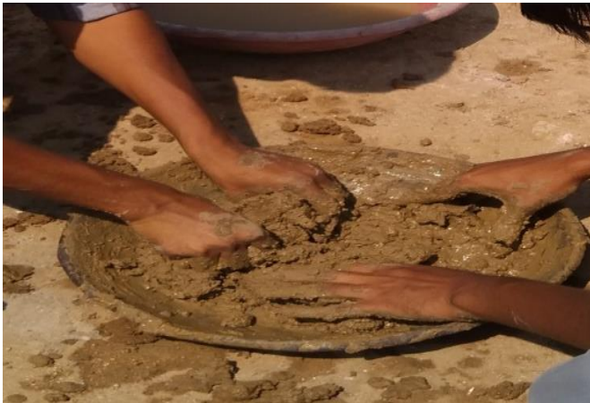
Fig:1 -Preparation Of Clay For Brick
