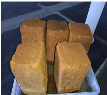
Fig:4- EFFLORSCENCE TEST ON ADMITURE ADDED BRICK
