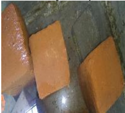
Fig:3-WATER ABSORPTION TEST ON ADMIXTURE ADDED BRICK
