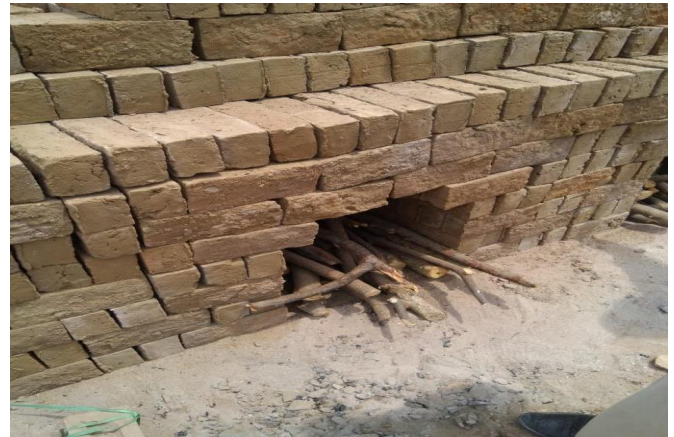
Fig:2-BURNING OF BRICKS
