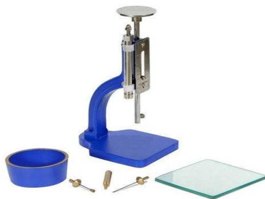
Fig. 1.1 Vicats Apparatus For Consistency And Initial, Final Setting Time
