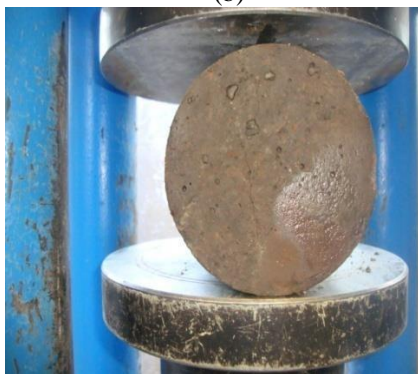
(b) Crack pattern Failure
