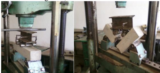
Fig 3: Flexure testing of beam.
