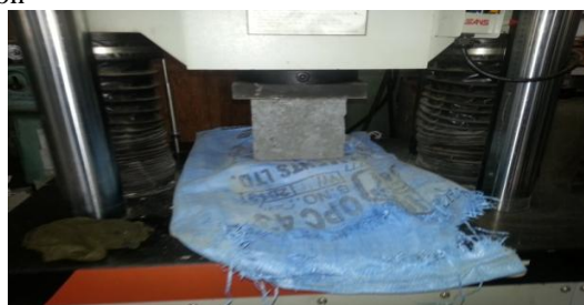
Fig 1 Compressive Strength Test Of Cube on UTM
