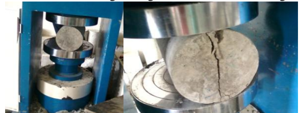
Fig 4: Loading arrangement for Split Tensile Strength Test.
