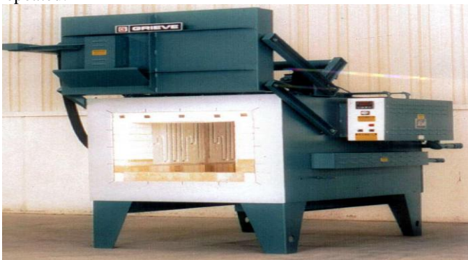
Fig : Electric furnace
