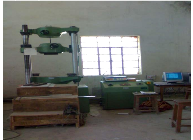
Fig: UTM testing setup
