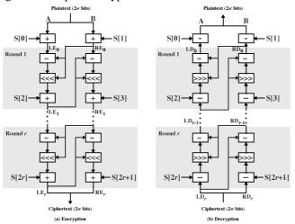
Fig 2 RC5 Encryption and Decryption
