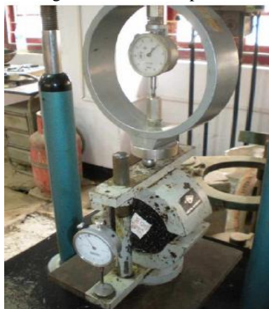
Fig 4: Marshall Test In Progress
