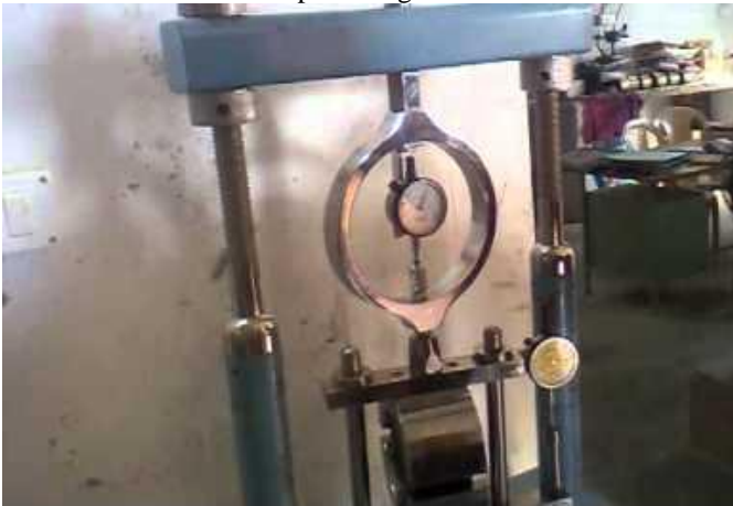
Fig 5: Marshall Stability testing of bituminous concrete specimen
