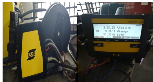
Fig 2.1: ESAB SSR 400-T Welding Setup.
