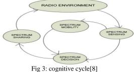
Spectrum sensing aims to determine spectrum availability and the presence of the licensed users. Spectrum management is to predict how long the spectrum holes are likely to remain available for use to the unlicensed users. Spectrum sharing is to distribute the spectrum fairly among the secondary users. Spectrum mobility is to maintain seamless communication during transition to better spectrum.
