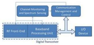
Fig 2: cognitive radio physical architecture.[8]
