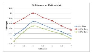
Fig 8 Variation of unit weight of BC with different binder content(With different fibre content)
