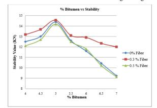
Fig 6 Variation of Marshall Stability of BC with different binder content (With different fibre content)
