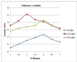
Fig 10 Variation of Stability Value of SMA with different binder content (With different fibre content)
