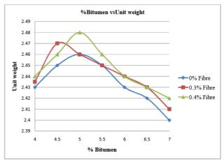
Fig 12 Variation of Unit Weight Value of SMA with different binder content (With different fibre content)
