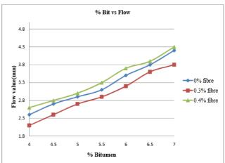
Fig 11 Variation of Flow Value of SMA with different binder content (With different fibre content)
