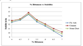
Fig 1 Variation of Marshall Stability of BC with different binder content
