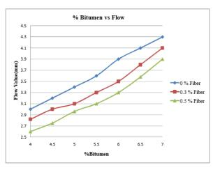
Fig 7 Variation of Flow value of BC with different binder content (With different fibre content)
