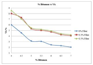
Fig 9 Variation of Air Void of BC with different binder content (With different fibre content)
