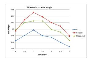
Fig 3 Variation of unit weight Value of BC with different binder content (With different type of filler)
