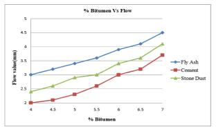
Fig 2 Variation of Flow Value of BC with different binder content (With different type of filler)
