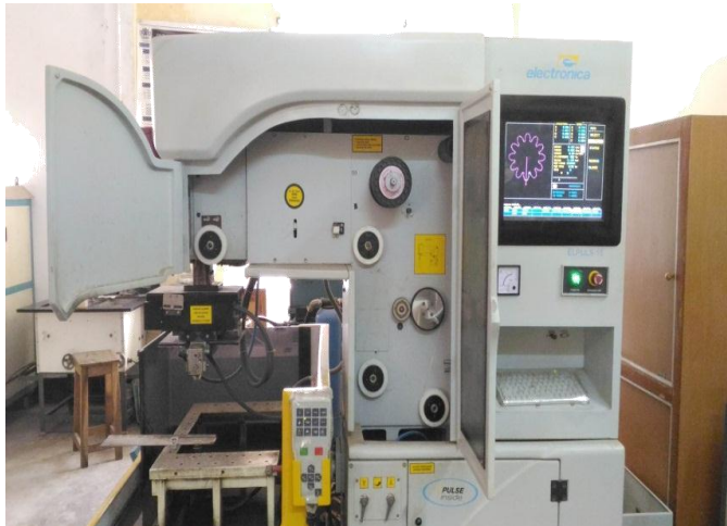
Fig. 1. Wire EDM machine setup cutting a gear
