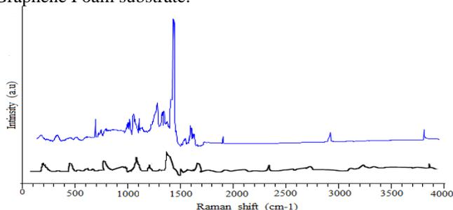
Figure 5. Comparison of SERS intensity of  $1\mu\text{M}$  MB on different SERS including Graphene Foam (black color) and AuNPs/GF (blue color).
