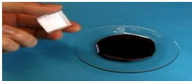
Fig. 10 Immerse the coating in a source of anthocyanins such as black grapes
