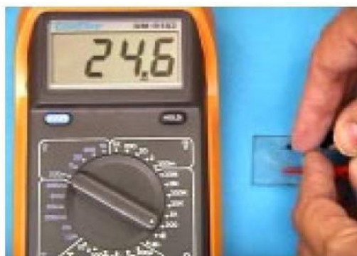
Fig 5 Identify the conducting side of glasses
