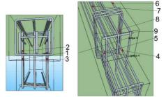
Fig. 6. Position of gauges in orthogonal reinforcement (M1).
