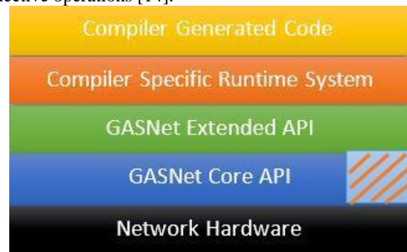
Fig. 3.3: GASNet Communication System
