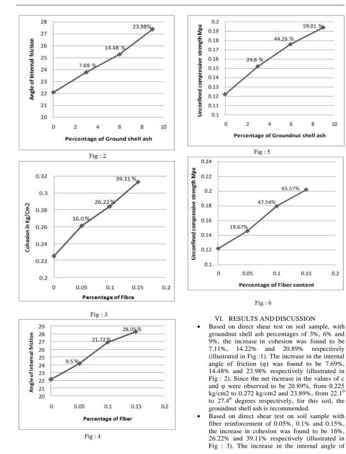
friction ( $\phi$ ) was found to be 9.5%, 21.72% and 28.05% respectively (illustrated in Fig : 4). Since the net increase in the values of c and  $\phi$  were observed to be 39.11%, from 0.225 kg/cm2 to 0.313 kg/cm2 and 28.05%, from 22.1<sup>o</sup> to 28.3<sup>o</sup> respectively, for this soil, randomly distributed polypropylene fiber reinforcement is recommended.
