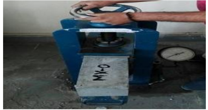
Fig. 2 TEST SET UP FOR BEAM
