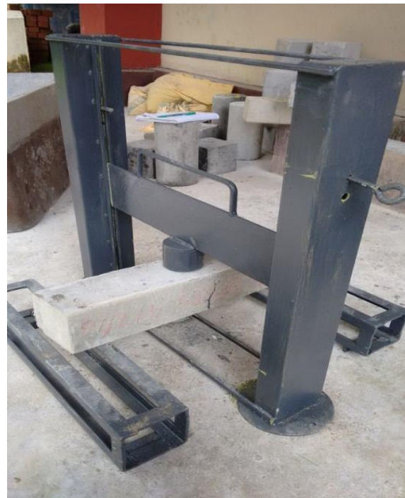
Fig. 1 Impact test rig with specimen
