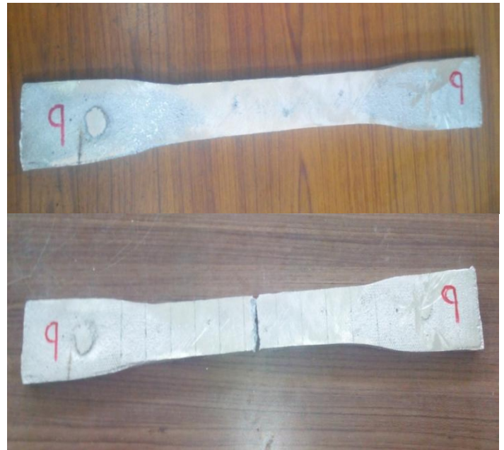
Figure 3: Tensile Test Specimen before and after the Test.
