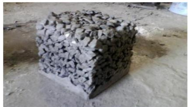
Fig. Specimen of Pervious Concrete
