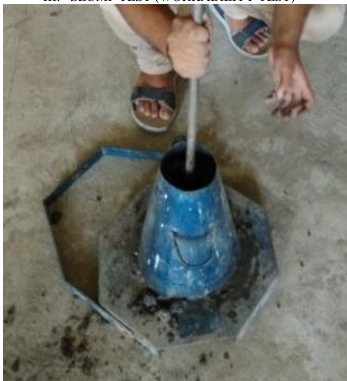
Fig. Process of Slump Cone Test
