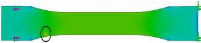
Figure 5. Von Mises Stress of a dogbone infected with a void.
