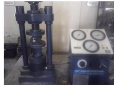
Fig. Cylinder specimen on compression testing machine
