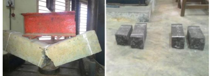
Fig.3.5 Beam specimens after testing for flexural strength
