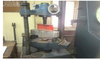
Fig.3.4 Beam specimen on universal testing machine (UTM)
