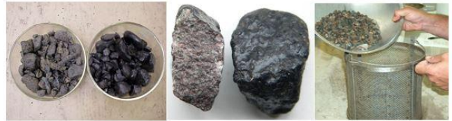
Fig.3.4 Stripping test of aggregate
