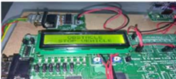
Figure: Output of ultrasonic sensor is displayed on LCD
