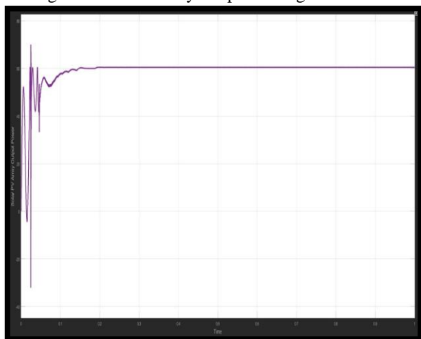
Fig.9- Solar PV Array Output Power
