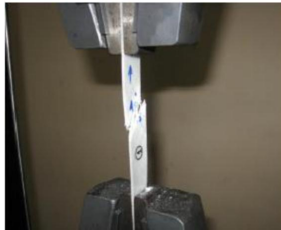
Figure 4.4: Failure pattern of woven fiber glass/epoxy composite specimen
