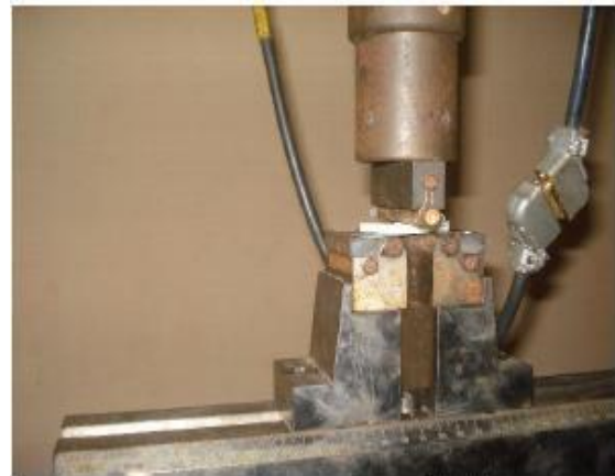
Figure 4.1 (a): Three point bend test setup and fixture
