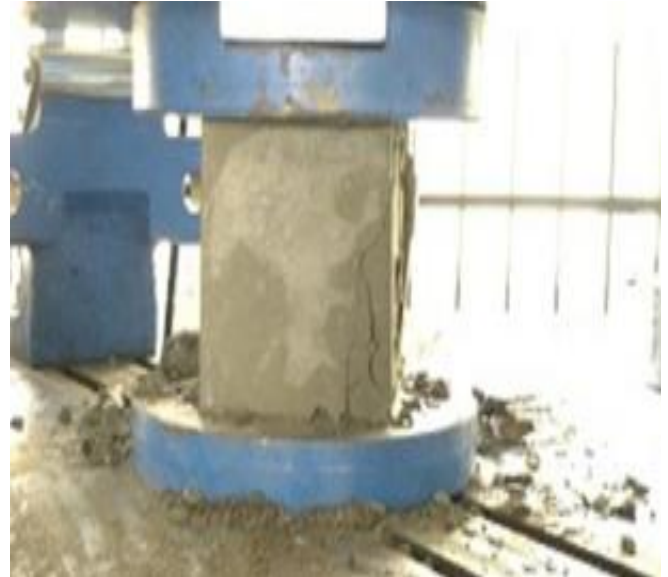
Figure: Compressive Strength test of cube samples in UTM aggregate size of 15mm
