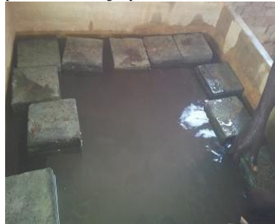
Figure: curing of samples
