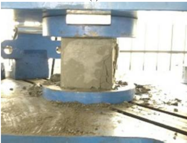
Figure: Compressive Strength test of cube samples in UTM of aggregate size of 3mm
