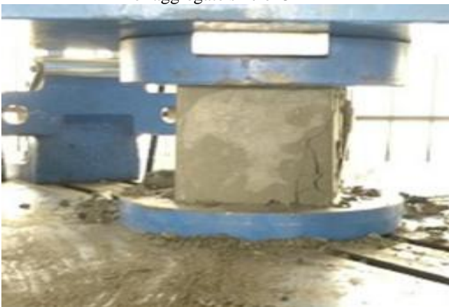
Figure: Compressive Strength test of cube samples in UTM aggregate size of 4mm
