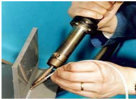
Fig. Hot gas hand welding[8]
