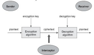
The illustration shows a sender who wants to transfer some sensitive data to a receiver in such a way that any party intercepting or eavesdropping on the communication channel cannot extract the data.
