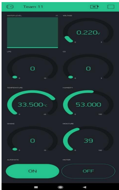
Fig.14: Motor turned OFF when moisture level is high.
