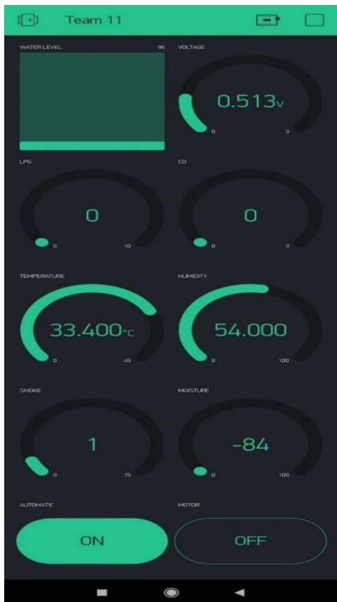
Fig.13: Motor turned ON when moisture level is low.
