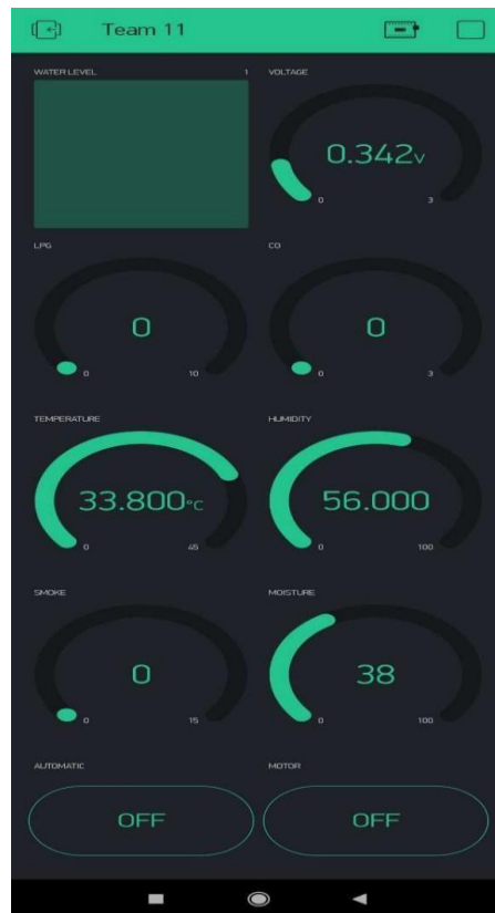
Fig.15: Motor Turned OFF with high moisture value
