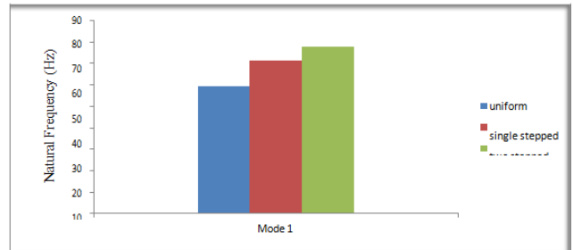
Figure 4.35: Plot of fundamental natural frequency (Hz) variation of uniform, single stepped and two stepped beams with respect to Mode1
