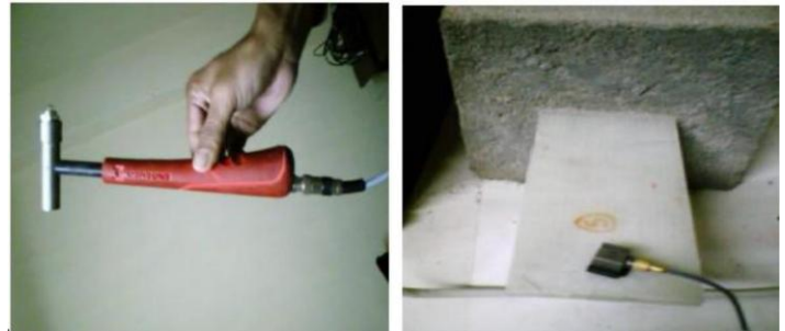
Figure 4.7: Modal Impact Hammer(type 2302-5) Figure 4.8: Accelerometer (4507)
