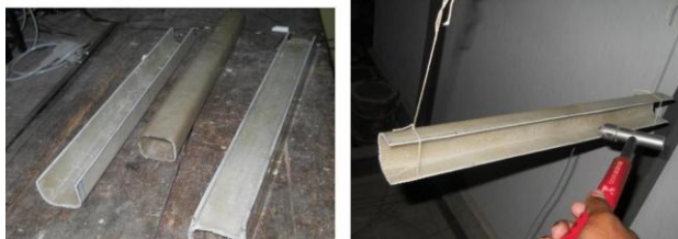
Figure 4.4: glass/epoxy composite specimen fabricated with different shapes
